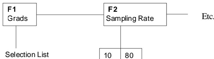
1. To move to a new heading, use the TARE (left) or ON/PRINT (right) key to move right or left in the Menu.
