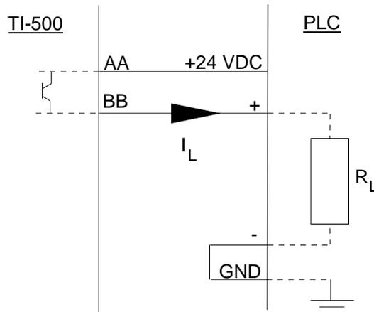
**NOTE 1:** Do NOT connect the indicator ground to the PLC ground.
