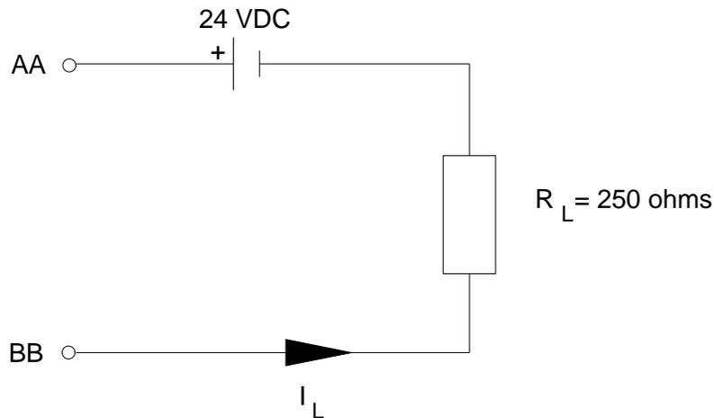
**NOTE 1:** In your application, substitute the actual input device for  $R_L$ . If your input device is polarized, connect the common lead to the negative lead of the 24 VDC power supply and the positive lead to the BB wire.
