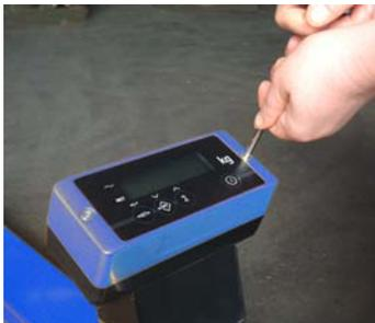
1. Remove the screws and then the indicator cover
