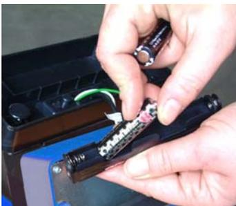
4. Place the new batteries in the battery holder
