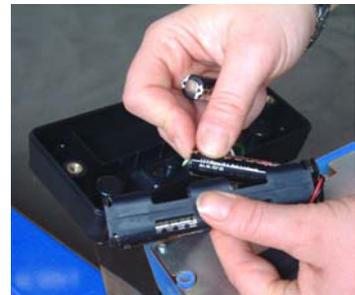
3. Remove the batteries from the holder
