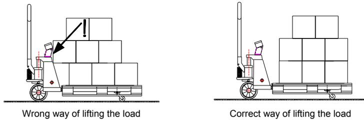
The accuracy of the weighing system diminishes with circa 0.1% per degree starting from a tilted position of 2°. This effect also occurs with pits/pot-holes in the floor. An even floor is optimal. The most accurate weighing result is obtained when the centre of gravity of the load is placed between the forks. With a non-centric loading, the forks will torque and bend. This may result in a higher inaccuracy.
