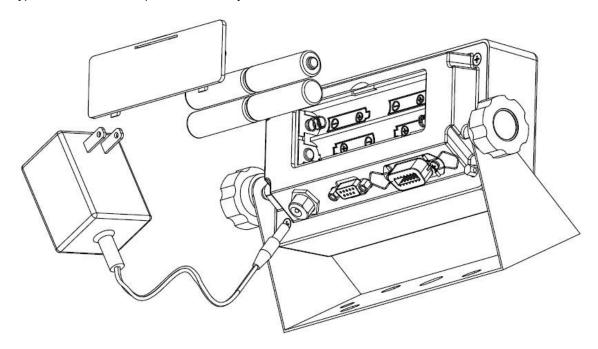
The TI-500 force data instrument may also be powered by the included AC wall adaptor included.
